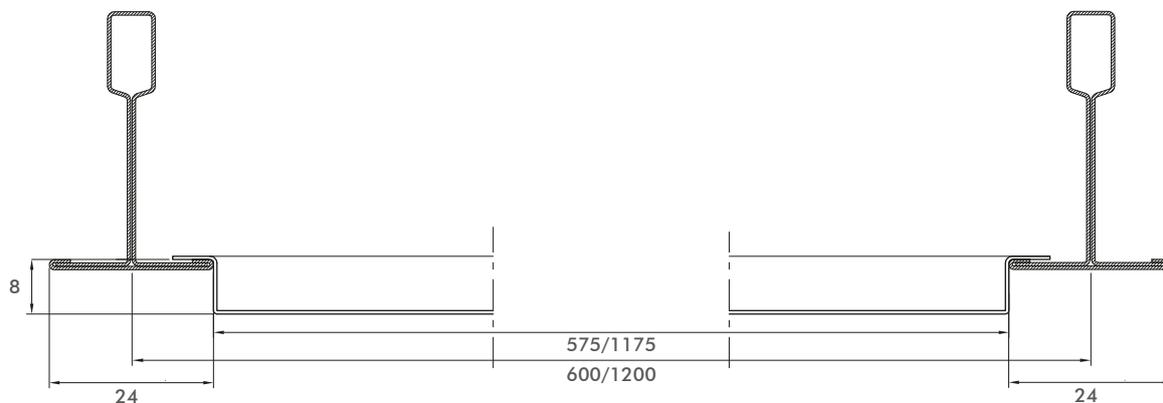
Sezione B - B' \_ on T24 structure \_ module 600x600 mm and 600x1200 mm
